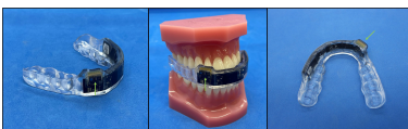
Figure 1. The buccal mucosal oximeter device. The photoplethysmography unit is indicated by the green arrows.
